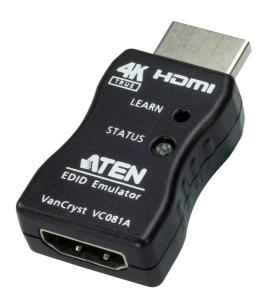
As a True 4K HDMI EDID Emulator Adapter, the VC081A is designed to emulate and store one set of the EDID from the connected display while facilitating 4K video transmission. By learning the EDID from the HDMI display and relaying it to the video source, the VC081A helps to eliminate video communication problems that occur due to the EDID data synchronization failure between the HDMI video source and the connected display.
