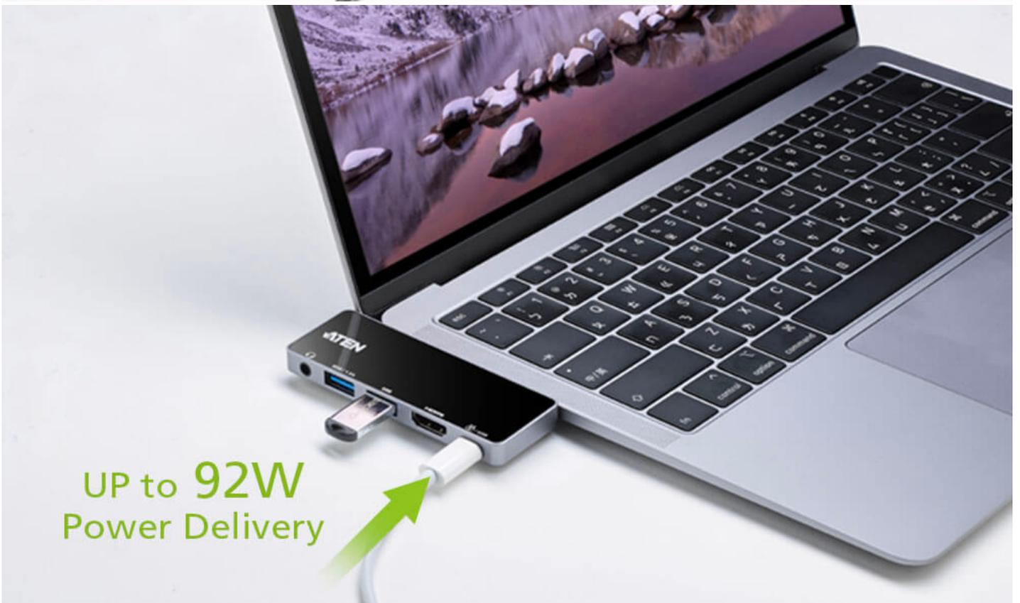
The USB-C port supports 92W power delivery providing full-speed pass-through charging for your Windows laptop, MacBook, Android tablet, iPad Pro, or smartphone, while also supporting standard 5Gbps data transfer.
