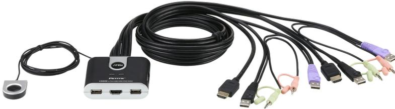
The CS692 2-Port USB HDMI/Audio Cable KVM Switch links two HDMI-enabled PCs or devices to a single USB keyboard, USB mouse, and HD display console. The CS692 Switch takes a giant step forward from prior cable KVM models in the Petite series, by offering full HDMI functionality, USB 2.0 peripheral sharing (via a USB hub attached to the USB mouse port), and a firmware upgrade function that allows you to keep up with latest available versions.
