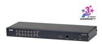
The KH1516A KVM switches are control units that allow IT administrators to access and control multiple computers from a single PS/2 or USB KVM console (keyboard, monitor, and mouse). Operators can take control of up to 16 computers. By daisy chaining up to 31 additional switches, as many as 512 computers can be controlled from the original KVM console.
