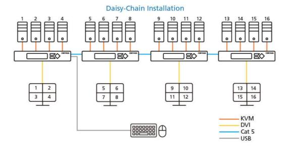
Furthermore, it can also be cascaded up to 2 levels by connecting additional 4 CM1164A units (up to 16 video sources) via a single console with video displayed in up to 4x4 multi-view mode.
