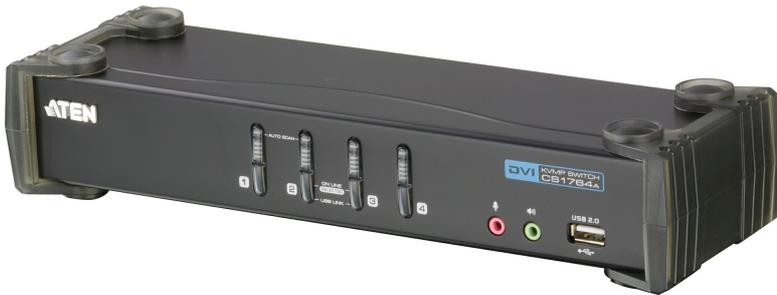
The CubiQ™ CS1764A USB 2.0 DVI KVMP™ Switch charts a revolutionary new direction in KVM (Keyboard, Video, Mouse) switch functionality by combining a 4-port KVM switch with a 2-port USB 2.0 hub at the same time as it provides an interface for a digital monitor (DVI).
