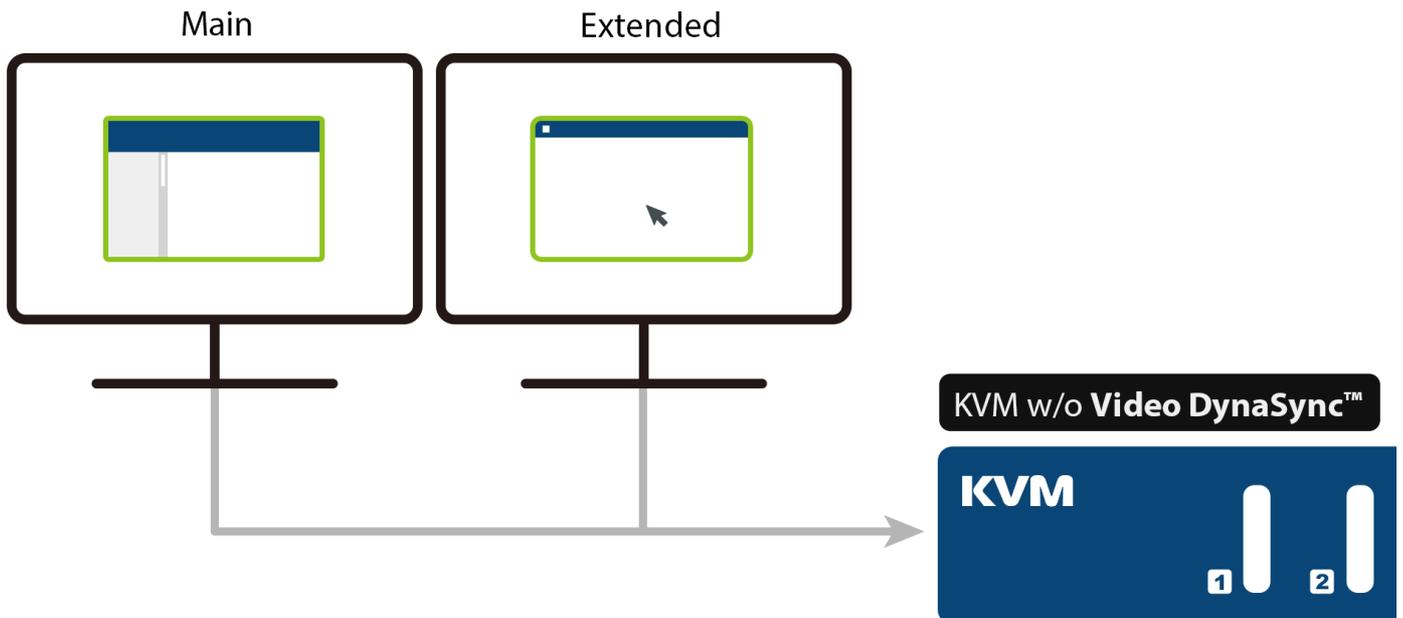
For requirements of more displays to monitor, users can daisy-chain two CS1844 for up to four displays to multitask easily and process tremendous information. Besides, a remote port selector is available for quick and streamlined port selection apart from pushbuttons, hotkeys and mouse port switching.
