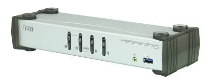
The ATEN CS1914 4-Port USB 3.0 DisplayPort <u>KVMP</u>™ Switch provides the latest innovations in desktop KVM switching technology to meet the increasing demand of higher video quality and file transfer rates on modern computers. The CS1914 provides superior resolutions up to 3840 x 2160 @ 30 Hz, a SuperSpeed USB 3.1 Gen 1 hub with 5 Gbps transfer rates and enhanced user-friendly operations.
