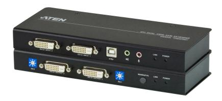
The CE604 is a DVI Dual View USB based <a href="KVM Extender">KVM Extender</a> that features Dual View functionality, which enables the video output to seamlessly display on two monitors. With RS-232 serial functionality, it allows access to a computer system from a remote console up to 60 m away. The CE604 is built for control and security purposes, and is targeted towards financial and industrial markets.
