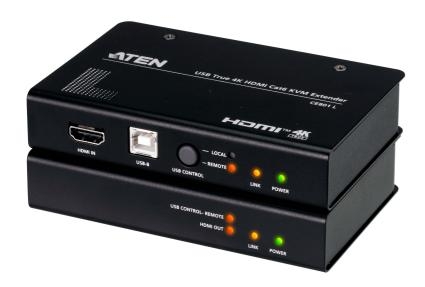
CE840 Extender kit enables sharp, life-like <u>True 4K</u> (4096 x 2160/3840 x 2160/@60Hz 4:4:4) HDMI, RS-232, and USB transmission across 70m over one single Cat 6 cable. It allows for dual console USB Keyboard/Mouse operation via the pushbutton for switching USB console control privilege between the remote and local units. RS-232 extension capability facilitates uninterrupted communication between serial-interfaced devices and equipment, which are still crucial in industrial control systems.
