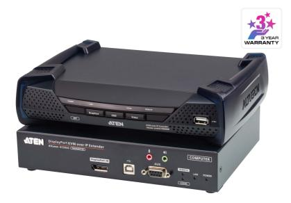
The KE9950 4K DisplayPort Single Display KVM over IP Extender consists of a high performance IP-based transmitter KE9950T that connects to the computer and receiver KE9950R that provides console access from a separate location. The KE9950 allows access to a computer system from a remote USB console (USB keyboard, USB mouse, DisplayPort monitor) over an intranet, enabling users to locate computers in a secure and temperature controlled environment, which is isolated from users' workstation.
