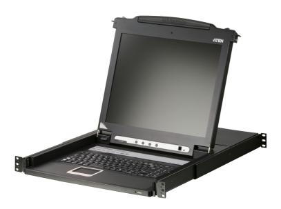
The CL1008\_<u>LCD KVM Switch</u> series are control units that allow access to multiple computers from a single keyboard, video, and mouse (KVM), console. A single CL1008 can control up to 8 computers. As many as 15 additional KVM switches can be daisy-chained to the CL1008, so that up to 128 computers can all be controlled from a single KVM console.
