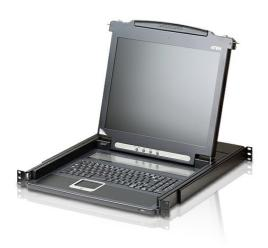
The CL1000 is a LCD KVM console that serves as the front-end for standard KVM switches. The CL1000 features an integrated 17" or 19" LED-backlit LCD panel, full keyboard, and touchpad in a 1U, rack-mountable, Slideaway™ housing.
