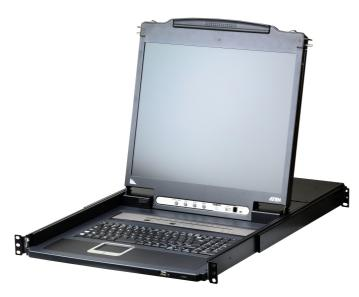
The CL5716I Slideaway<sup>™</sup> <u>LCD KVM Switch</u> is a control unit that allows access to multiple computers from a single PS/2 or USB KVM (keyboard, video, and mouse) console. A single CL5716I can control up to 16 computers. As many as 15 additional KVM switches can be daisychained to the CL5716I, so that up to 256 computers can all be controlled from a single KVM console.
