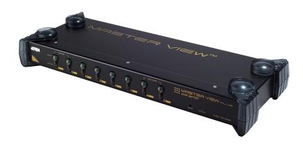
CS9138 is a high-efficiency KVM Switch which provides the most efficient solution to fulfill the management needs of server networks. It is a KVM Switch with 8 ports and can control 8 computers. It allows connections in 3 tiers by cascade. With 73 sets of CS9138, users can connect up to 512 servers.
