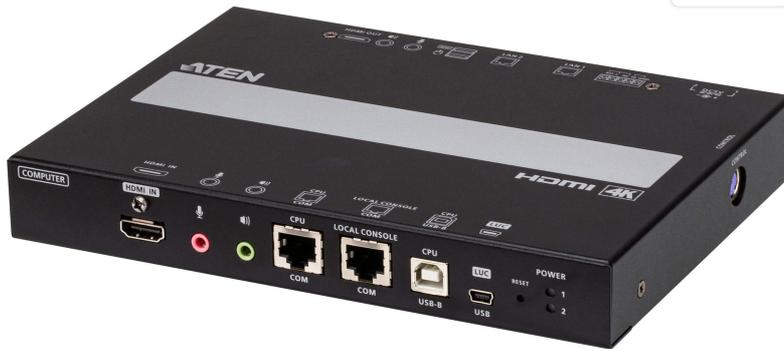
The RCMHD101U Single Port HDMI KVM over IP Switch is a KVM device exclusively designed for production line applications, which can grant the video, audio, mouse & keyboard, and [virtual media](#) access of a workstation at a production line to a local and remote consoles for convenient management. It also supports microphone and speakers for both local and remote consoles.
