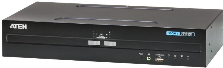
ATEN [PSS PP v3.0 Secure KVM](#) Switch (CS1142H) is specifically designed to meet the stringent security requirement of secure defense and intelligence installations. ATEN [PSS PP v3.0 Secure KVM](#) Switch (CS1142H) is compliant with [PSS PP v3.0](#) (Protection Profile for Peripheral Sharing Switch, Version 3.0) standard certified by the National Information Assurance Partnership (NIAP).
