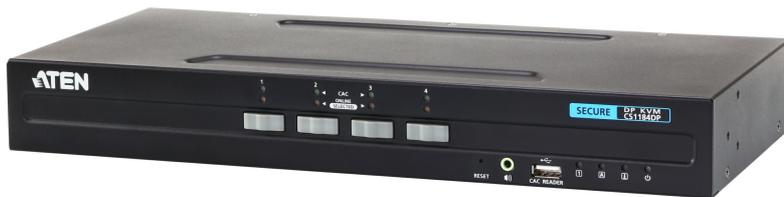
ATEN [PSS PP v3.0 Secure KVM](#) Switch (CS1184DP) is specifically designed to meet the stringent security requirement of secure defense and intelligence installations. ATEN [PSS PP v3.0 Secure KVM](#) Switch (CS1184DP) is compliant with [PSS PP v3.0](#) (Protection Profile for Peripheral Sharing Switch, Version 3.0) standard certified by the National Information Assurance Partnership (NIAP).
