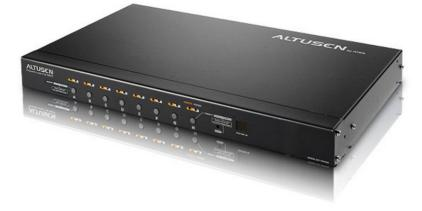
The PN9108 Power over the NET<sup>™</sup> is a control unit that provides remote power management for eight AC outlets via a TCP/IP connection, allowing administrators to control the power off, power on, and reboot status for each attached device from any computer connected to the Internet, whether down the hall, or half way around the world. The PN9108 is the most convenient, reliable and cost effective way to obtain access to your server room remotely.
