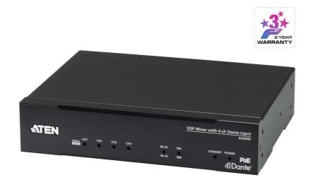
The AD004E converts Dante inputs into 4-channel analog line outputs, integrating analog and digital audio devices into one single system through Dante AoIP media networking technology. This SHARC® ADSP-21489 processor embedded device supports 24 bit and offers sampling rate options of 44.1k, 48k, 88.2k, and 96 kHz, delivering advanced audio processing to meet commercialgrade application needs
