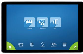
The ATEN VK320 is an 8" Touch Panel featuring capacitive multi-touch IPS-LCD screen with a narrow bezel. Natively installed with the <a href="ATEN Control System">ATEN Control System</a> app, the touch panel is compatible with ATEN Control Boxes and Control Pads.
