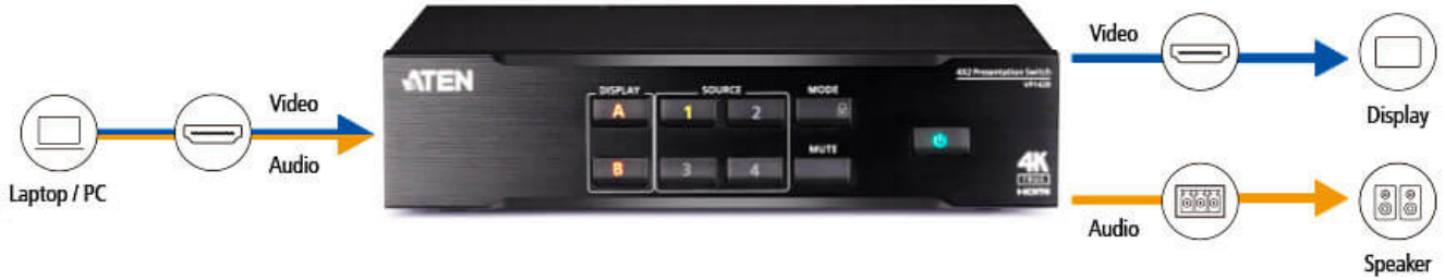
Audio De-embedding Extract HDMI audio to Audio Line Out
