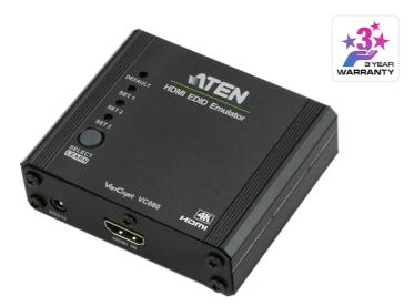
The ATEN VC080 is a HDMI EDID Emulator, which is designed to emulate and store the EDID of a video display, providing constant and reliable EDID data for the a HDMI source device to efficiently optimize video resolution.
