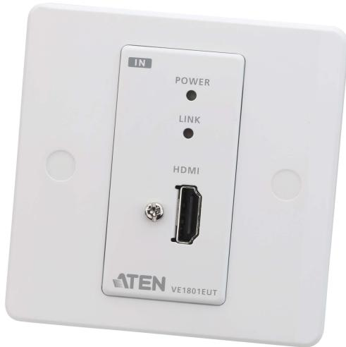
ATEN VE1801EUT is a transmitter designed to reliably send 4K signals up to 40 m over a single Cat 5e/6/6a or ATEN [2L-2910](#) Cat 6 cable. With EU Wall Plate design, the VE1801EUT can be conveniently mounted in a one-gang junction box. For HDMI signal transmission, it supports 3D, Deep Color, and embedded HD lossless audio formats.
