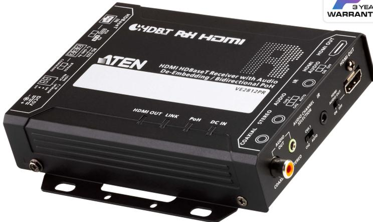
Featuring powerful Class A HDBaseT technology, the VE2812PR is a receiver for 4K HDMI video, audio, and control signals over a distance of up to 100 m via a Cat 5e / 6 / 6a or ATEN [2L-29330](#) Cat 6 cable. HDMI signal transmission extends further up to 150 m @ 1080p when the HDBaseT Long Reach Mode is enabled.
