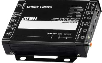
The VE2812R is a high-quality HDMI HDBaseT Receiver featuring audio de-embedding function. Powered by HDBaseTTM technology, the VE2812R can receive 4K HDMI signals up to 100 m over a single Cat 5e/6/6a or ATEN 21-2910 Cat 6 cable. With HDBaseT Long Reach Mode enabled, it can deliver HDMI signals up to a maximum range of 150 meters @ 1080p.
