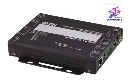
The ATEN VE3912T is an HDBaseT transmitter that extends 4K DisplayPort, HDMI, or VGA video signals up to 100 m over a single Cat 6/6a or ATEN 2L-2910 Cat 6 cable. Featuring multiple video input formats and output resolutions up to 4K, it ensures a superior video quality for applications that require digital/analog sources conversion and extension.
