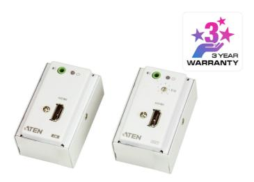
The VE807 HDMI/Audio Cat 5 Extender with MK Wall Plate is designed to be conveniently mounted in a one- gang junction box for the UK, Singapore, Hong Kong and other markets that apply MK type junction boxes. It extends HDMI and audio signals up to 60 meters over a Cat 5e/6 cable and supports widescreen formats ensuring excellent video quality.
