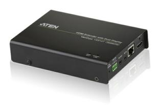
Place your HDMI displays up to 100 meters away from your HDMI source devices with the VE814T HDMI Transmitter over single Cat 5 with Dual Display. Connecting to the VE814R receiver via affordable and easily available Cat 5e/6 cable, your media can be streamed to up to three HDMI displays – dual displays connected to the receiver and another to the transmitter.
