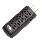
The VE819T HDMI Dongle Wireless Transmitter is an ideal choice for meeting rooms and home theater systems. It sends uncompressed Full HD 1080p signal from your HDMI devices such as laptops, computers and set top boxes. Up to four Wireless HDMI Transmitters can be paired to the Receiver, boosting the number of total transmitters per receiver to a maximum of 4.
