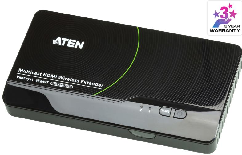
The VE849T Multicast HDMI Wireless Transmitter allows you to position HDMI displays up to 30m\* away from HDMI sources when used in unison with up to 4 [VE849R](#) receivers.
