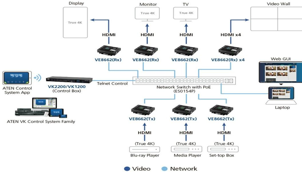
Note: VE8662 supports PoE and can be installed in combination with PoE network switches to reduce power cabling and additional power outlets. Before choosing the Network switch and installation, please refer to the Implementation Guide.
