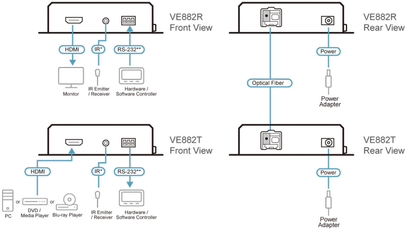
\* The IR bypass channel is bi-directional. The IR transmitter and IR receiver can be plugged either into the VE882T or VE882R unit depending on the device you want to control remotely.
