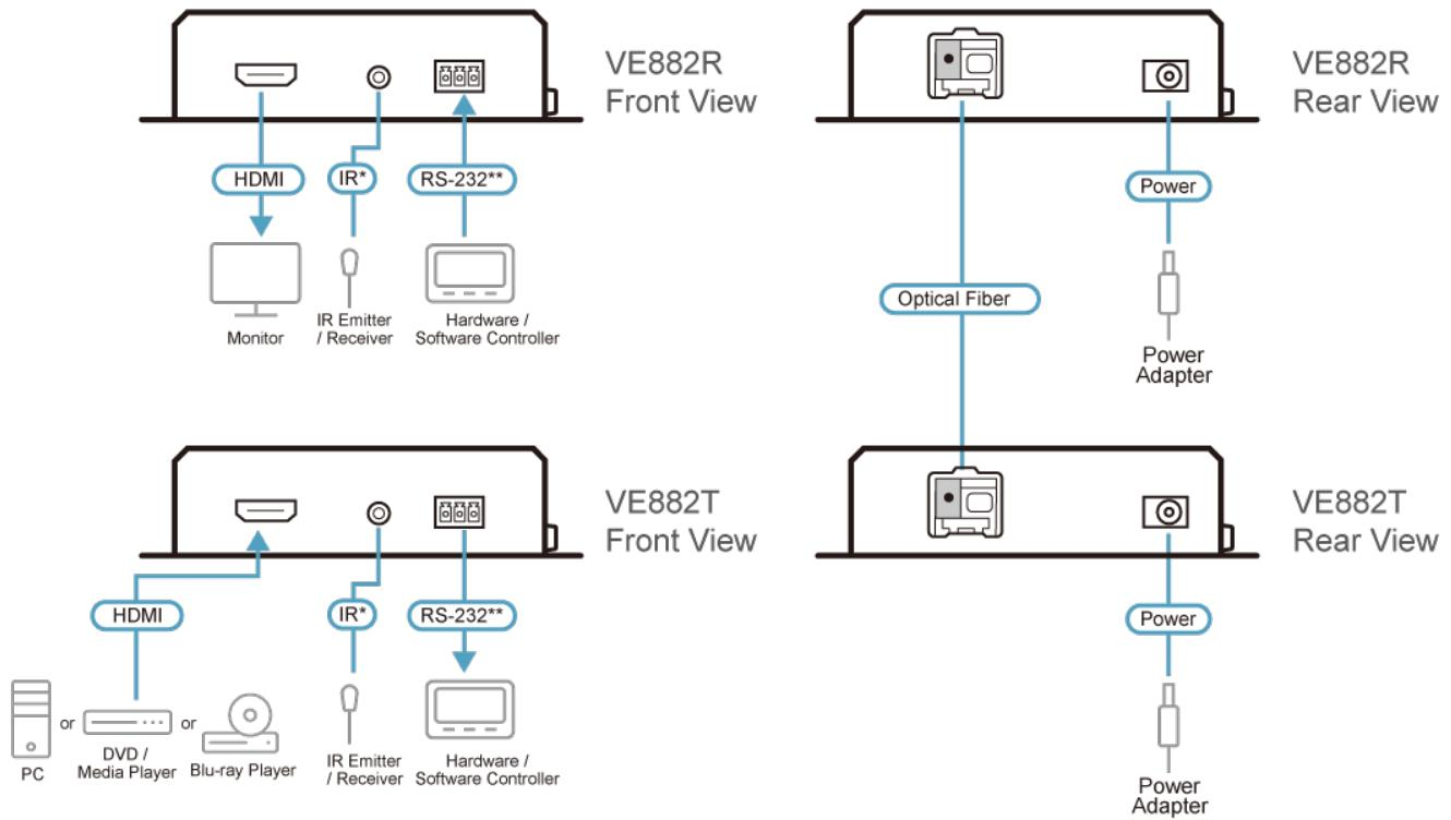
\* The IR bypass channel is bi-directional. The IR transmitter and IR receiver can be plugged either into the VE882T or VE882R unit depending on the device you want to control remotely.
