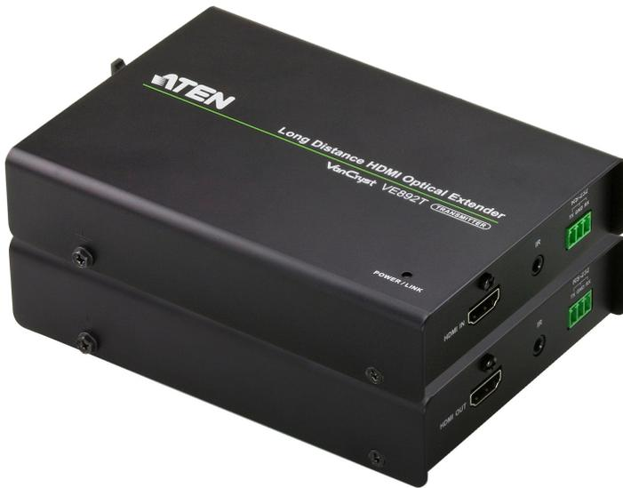
The VE892 is an Optical HDMI Extender that overcomes the length restriction of standard HDMI cables by using optical fiber to send high definition audio and video signals over large distances.
