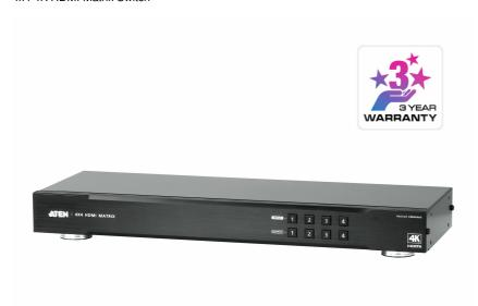
The ATEN VM0404HA 4x4 4K HDMI Matrix Switch supports 4K resolutions of UHD (3840 x 2160) and DCI (4096 x 2160) with refresh rates of 30 Hz (4:4:4) and 60 Hz (4:2:0). Ready for the future of highdefinition video switching, the VM0404HA is ideal for applications where the routing of 4K digital signals is required, such as in classrooms, auditoriums, department stores and more.
