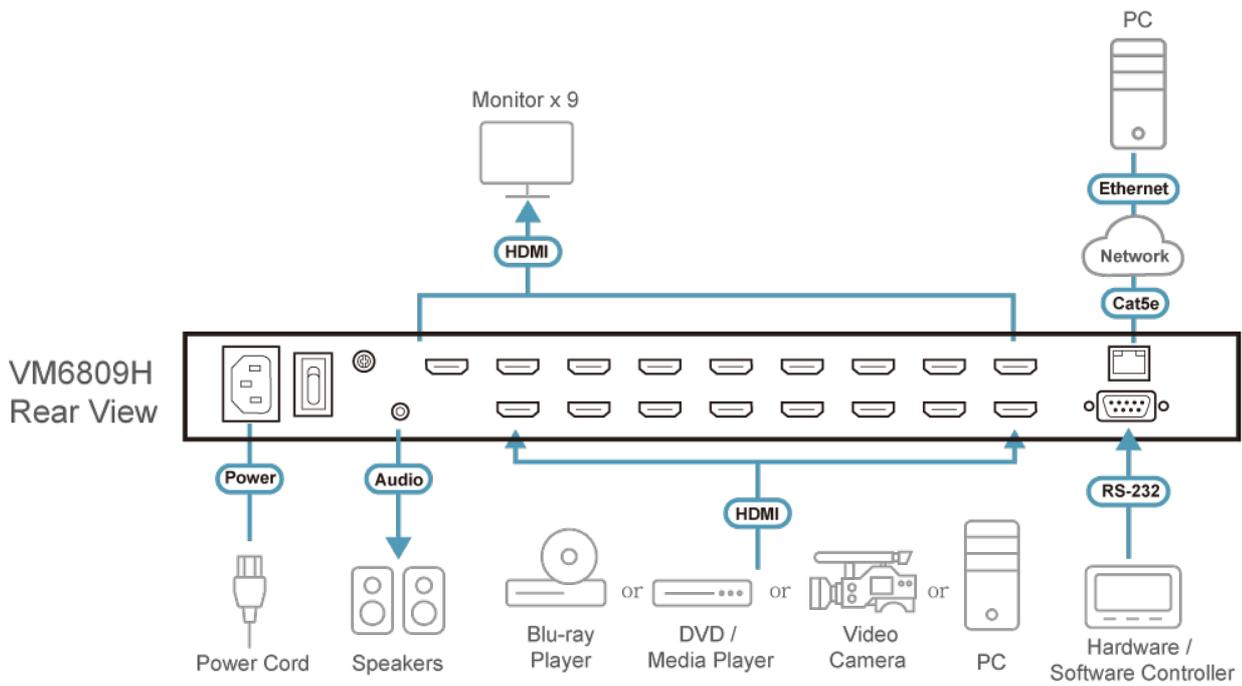
Note: Connects up to 9 display devices to the HDMI output ports, and up to 8 video source devices to the HDMI input ports.
