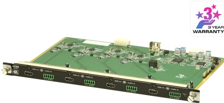
The VM7814 is a 4K HDMI input board that works with an ATEN [Modular Matrix Switch](#) to offer an easy way to route 4 HDMI sources to 4 displays. In addition to the HDMI interface that carries digital A/V signals, the VM7814 is equipped with 4 stereo audio input ports that allow stereo audio embedding.
