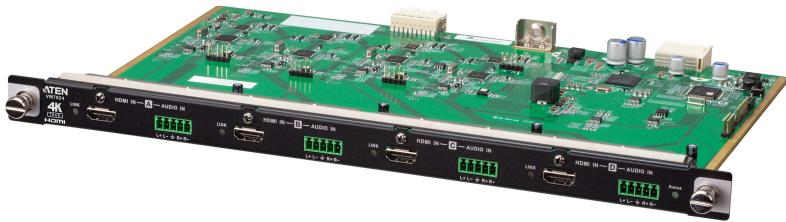
The VM7824 is a True 4K HDMI input board that works with an ATEN [Modular Matrix Switch](#) to offer an easy way to route 4 HDMI audio/video sources to 4 displays with True 4K high-definition images support. In addition to the HDMI interface that carries digital A/V signal, the VM7824 also provides 4 stereo audio input ports that enable stereo audio embedding.
