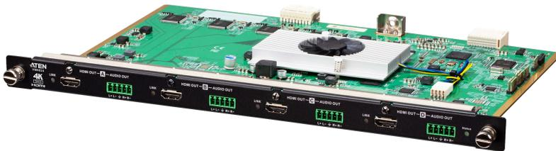
The VM8824 is a True 4K HDMI output board that works with an ATEN [Modular Matrix Switch](#) to offer an easy way to route 4 analog/digital audio/video sources to 4 HDMI displays with True 4K high-definition images support. In addition to the HDMI interface that carries digital A/V signal, the VM8824 also provides 4 stereo audio output ports that enable HDMI audio extraction.
