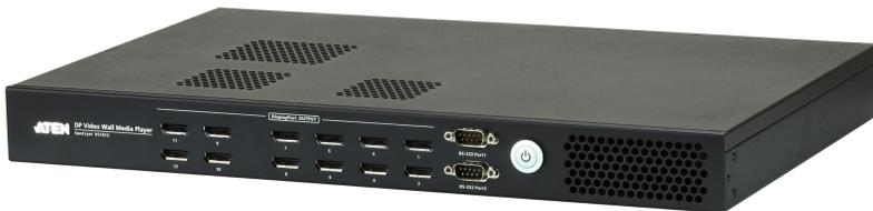
The VS1912 12-Port DP Video Wall Media Player is a PC-based media player and an ideal solution for multi-display applications such as digital signage, video walls, projection screens and digital board installations.
