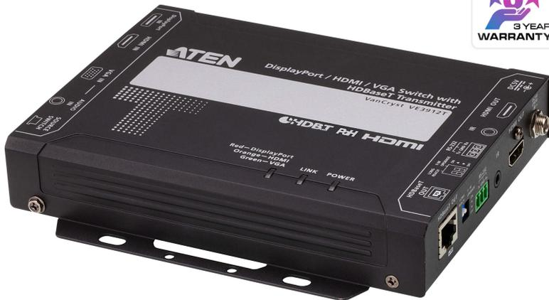
The ATEN VE3912T is an HDBaseT transmitter that extends 4K DisplayPort, HDMI, or VGA video signals up to 100 m over a single Cat 6/6a or ATEN [2L-2910](#) Cat 6 cable. Featuring multiple video input formats and output resolutions up to 4K, it ensures a superior video quality for applications that require digital/analog sources conversion and extension.
