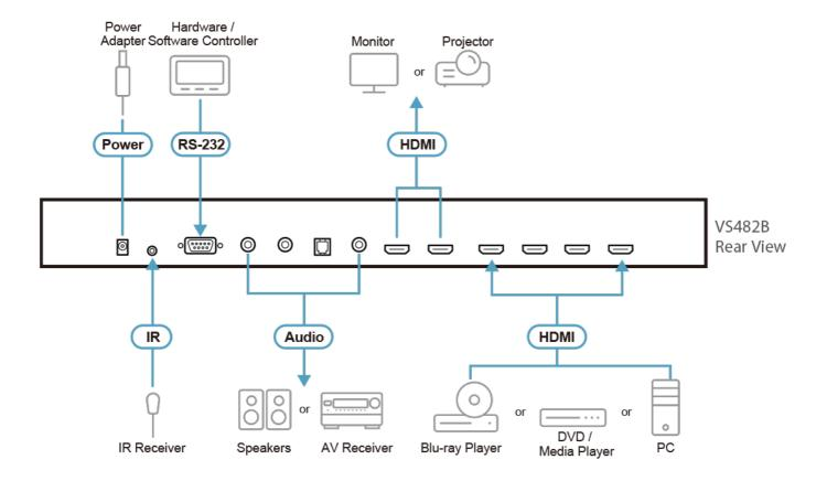
Note: Connects up to 2 display devices to the HDMI output ports, and up to 4 video source devices to the HDMI input ports.
