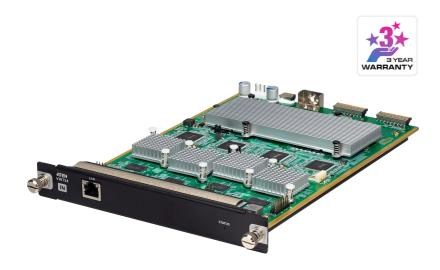
Built to work with ATEN's <u>VW3620</u> Modular Video Wall Processor, the VW754 seamlessly accepts H.265/H.264 streams from IP cameras/Network Video Recorders (NVRs) and decodes up to four channels at 4K @ 60 Hz simultaneously. Each decoded stream is assignable to a preferred output channel within the <u>VW3620</u> configuration\*. The VW754 facilitates seamless integration with any mainstream IP-based video system on account of its compliance with ONVIF Profile S and the support for RTSP.
