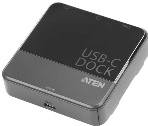
The ATEN UH3233 is a [USB-C](#) Dual-HDMI Mini Dock which transforms your [USB-C](#) device to a dual monitor workstation. It's compliant with the latest USB 3.1 Type-C specifications and supports dual display mode. The UH3233 can route video from the source device to two HDMI monitors, splitting the video transmission for a dual-view display via a single cable while maintaining a high quality resolution up to 1080p.
