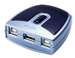
US221 allows 2 computers to share the same USB peripheral under the foundation of one-at-a-time. Users can switch the computer controlling the peripheral from the simple hotkeys or buttons on the front panel or the control software on Windows. It is ideal for SOHO environments. 20050223153137004.jpg
