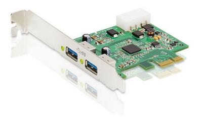
ATEN IC320 is a 2-port USB 3.0 PCI-e Card, which supports USB 3.0 Super-Speed devices. It provides speeds of up to 10x faster than that of USB 2.0, enabling you to access and transfer your data much faster simply by adding two USB 3.0 ports to your PCI Express-capable PC. It is backwards compatible with USB 2.0 and USB 1.1, ensuring compatibility with existing devices.
