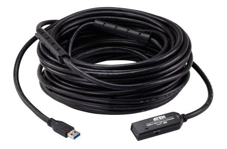
The UE332C is a USB 3.2 Gen 1 extender cable for adding 20 m to the connection between a USB Type-A enabled PC / laptop and a USB-C device. With the support of up to 5 Gbps Super Speed data transfer rates, the UE332C is backward compatible with USB 2.0 and 1.1 standards, ensuring reliable data communication.
