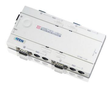
CS14 is a KVM switch with built-in PS/2. It can control 4 servers via a single console and allows users to switch between computers via the buttons on the upper part of the switch or the hotkey configuration on the console keyboard. It is the simplest and most convenient most convenient solution for multi-computer management.
