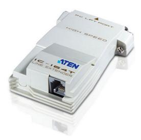
The IC164 parallel signal extender can extend the distance between your parallel peripherals and the PC up to 400m, thus allowing you to control parallel peripherals from far away. The local unit and remote unit of IC-164 are connected with the RJ-11 cable, which is easy and time-saving to install.
