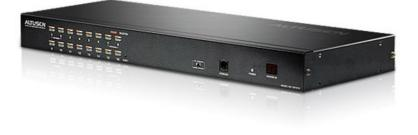
The KH1516 KVM Switches are control units that allow access to multiple computers from a single KVM (keyboard, monitor, and mouse) console. The KH1516 features RJ-45 connectors and Cat 5e/6 cable to link to the computers. Combined with Auto Signal Compensation (ASC) signals can travel up to 40 meters and still maintain high video resolution.
